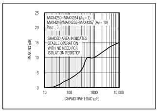
Figure 7. Peaking vs. Capacitive Load
