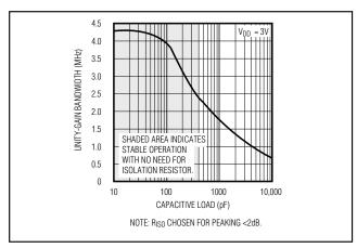
Figure 8. MAX4250-4254 Unity-Gain Bandwidth vs. Capacitive Load
