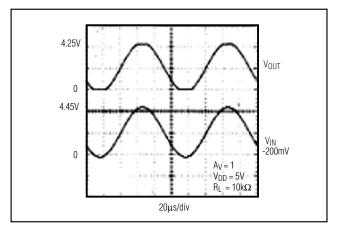
Figure 4. Rail-to-Rail Output Operation
