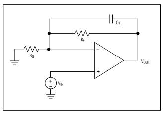
Figure 1. Adding Feed-Forward Compensation
