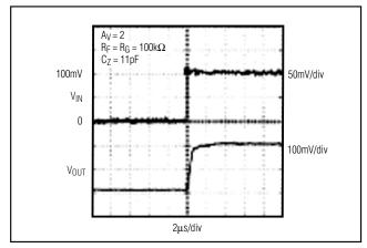
Figure 2b. Pulse Response with 10pF Feed-Forward Compensation
